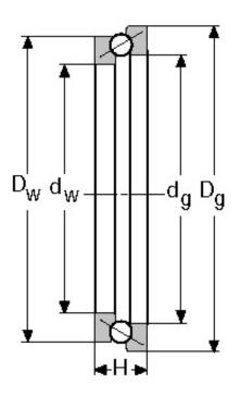
**MONTON** single direction angular contact thrust ball bearings can be supplied in matched sets of two, three or four bearings.
