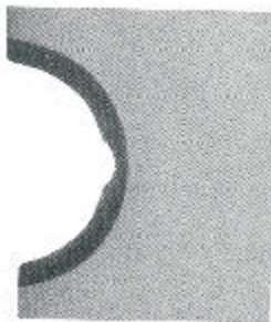
Raceway of single row four-point contacted ball bearing
