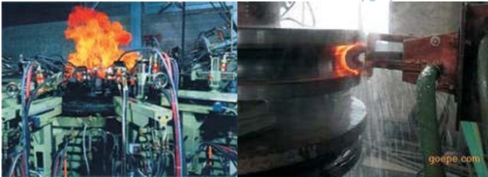
Sketch of raceway nest quenching
