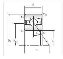
MONTON B719XX extremely light Series Angular Contact Ball Bearings diameter from 10-670
