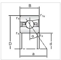
MONTON B72XX robust Series angular contact ball bearings size from 10mm-400 mm. B72 series bearings have a large
