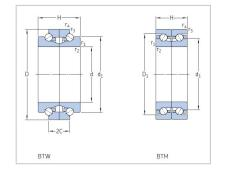
MONTON double direction angular contact thrust ball bearings are designed to locate spindle shafts in both directions. These bearings combination with cylindrical roller bearings in the NN 30 K or N 10 K series in the same housing bore. This bearing combination simplify machining of the housing bore.
