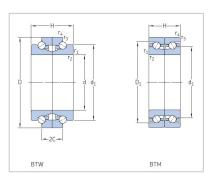
MONTON double direction angular contact thrust ball bearings are designed to locate spindle shafts in both directions. These bearings combination with cylindrical roller bearings in the NN 30 K or N 10 K series in the same housing bore. This bearing combination simplify machining of the housing bore.
