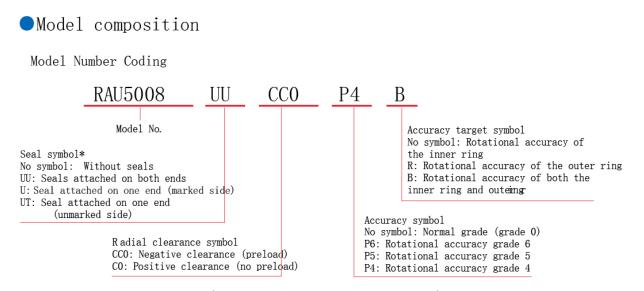
Considerations for model RAU (Small-diameter thin type. Width: 5mm) \*Seals are not available.\* The omdyar clearance available is CO.\* The only accuracy available is normal grade (grade 0). [Micro Cross-Roller Ring with inner diameter of 10 mm and outer diameter of 21 mm
